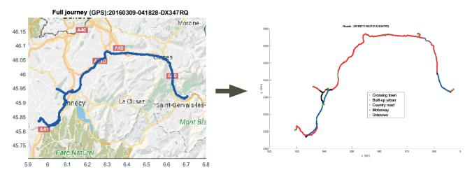
Note that some sections have not been categorised (marked in green in the diagram on the right). These are sections in which the vehicle was manoeuvring or sections affected by mapping problems. These sections were not included in the analysis.
